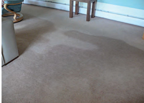
ABOVE: Carpet pile responds to foot traffic sometimes in ways which appear quite random, in this case, “shading”, which is a normal characteristic of cut-pile carpet.
