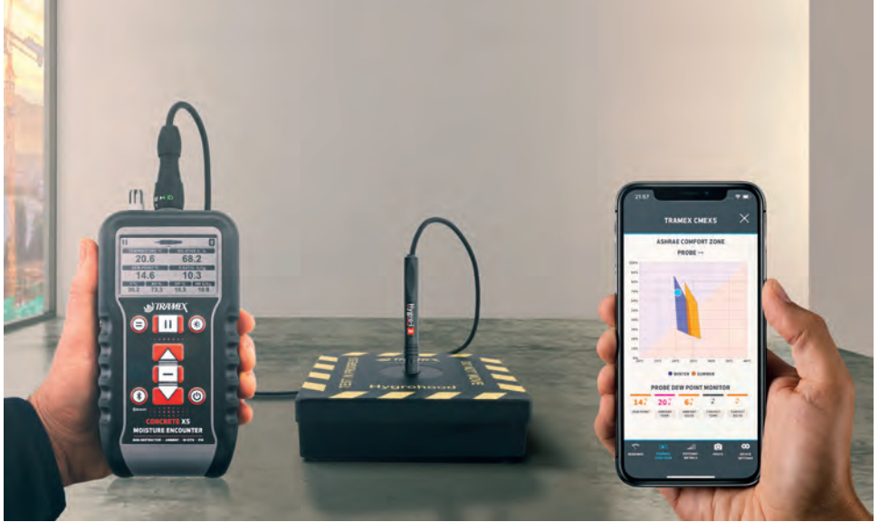
ABOVE: Tramex CME5, Hygrohood, RH probes for relative humidity and moisture content testing of concrete and anhydrite floors and screeds; ambient temperature and relative humidity; Bluetooth connectivity to the Tramex Meters App. Visit www.tramexmeters.com
