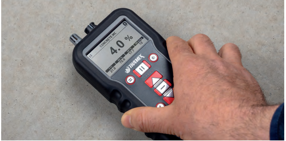
ABOVE: Tramex CME5 for instant, non-destructive and quantitative %MC moisture content testing of concrete and anhydrite floors and screeds; ambient temperature and relative humidity; Bluetooth connectivity to the Tramex Meters App. Visit www.tramexmeters.com
